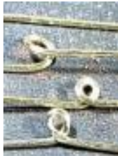
Top, straight wire, casual loop in wire, eye pulled tight on pin, eye flattened with pliers.
