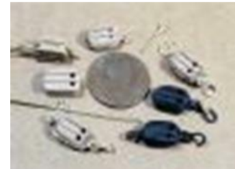
From block blank on far left to wire stropping and hooks. All wire joints are soldered. Hook eyes will be soldered after they are in block eyes.
