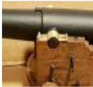
Fitting the cap squares to the cannon carriage awaiting staple and pin that will hold it in place.
