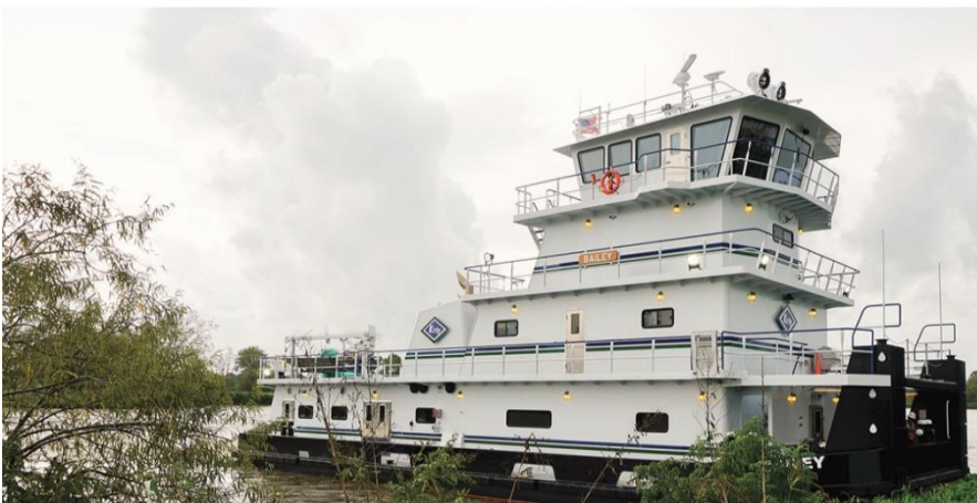
Main Iron Works owner Arlen “Benny” Cenac Jr. recently announced completion of the first of three 2,680 hp. towboats the shipyard is building for Kirby Inland Marine . The vessel, named the mv. Bailey, is a Sterling Marine design and measures 88 feet by 35 feet, with a molded depth of 12 feet 2 inches and a draft of 9 feet.
